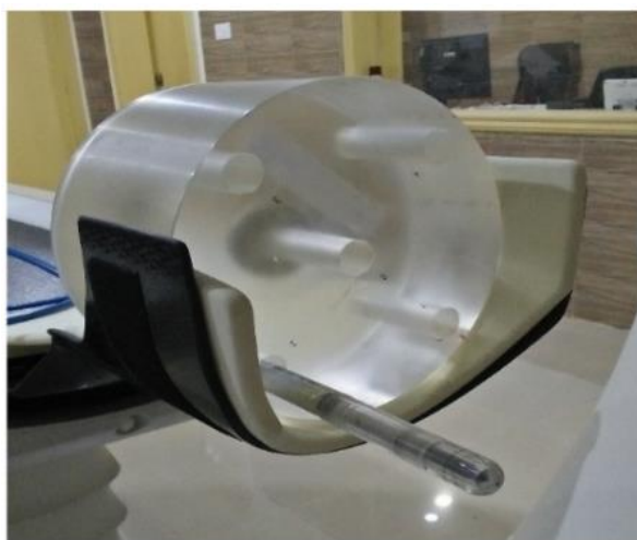
Figure-1: Solid PMMA cylindrical phantom (Krieger T9193) used as a CT head phantom.
