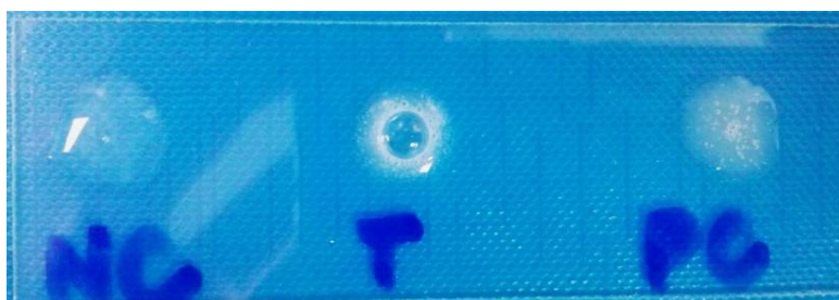
Figure 3. 5: Proteus mirabilis was catalase-positive and metabolized H_2O_2
