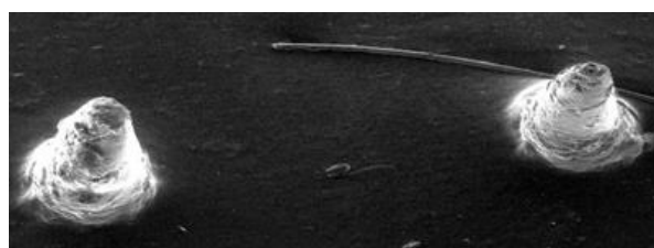
Figure 8: Measurement of the space between two needles by scanning electron microscopy
