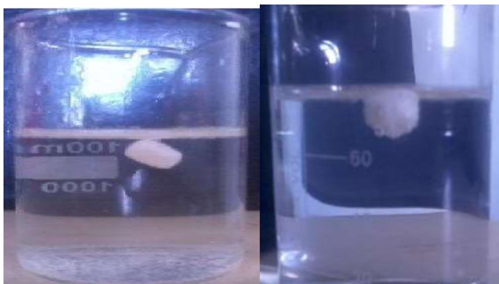
Fig 15 In-vitro buoyancy studies of the Glipizide floating tablet using Sodiumalginate (F4)
