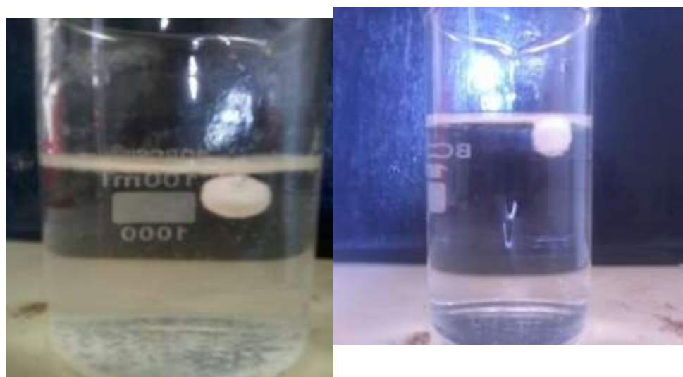
Fig 15 In-vitro buoyancy studies of the Glipizide floating tablet using Sodiumalginate (F4)
