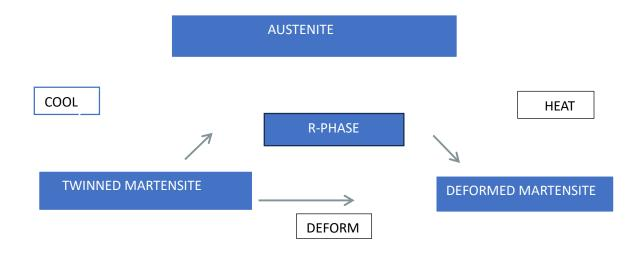
Nickel-titanium alloys demonstrate the shape memory effect, wherein they revert to their original shape from the martensitic phase upon heating or when stress is relieved.
