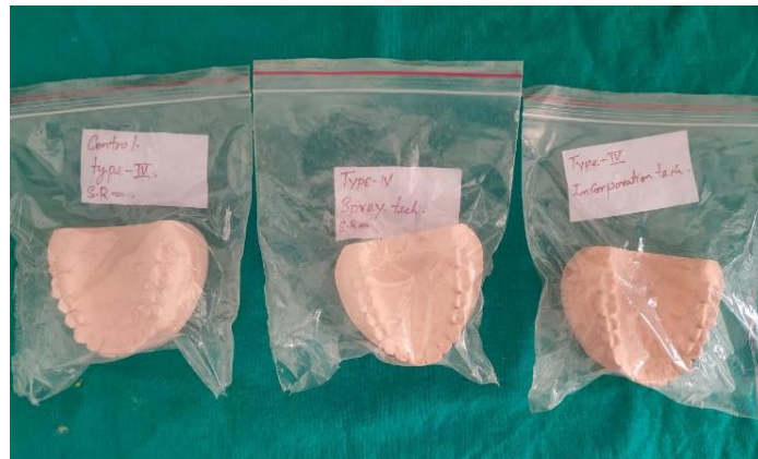
Figure 1- Samples stored in zip lock bag after disinfection prior to material testing
