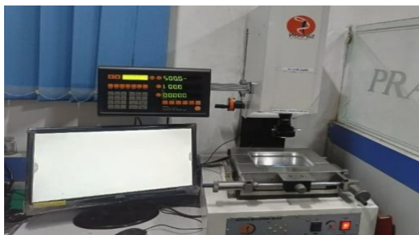
Figure 4- Measuring surface roughness using contact profilometer Figure 5- Measuring dimensional stability using vision inspecting system
