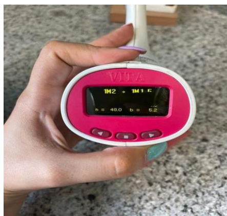
Figure 4. Color matching of samples with VITA Easyshade
