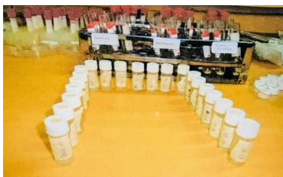
Figure 3: Fluoride Ion Eluates in Chromatography Vials Prior to IC Quantification Results
