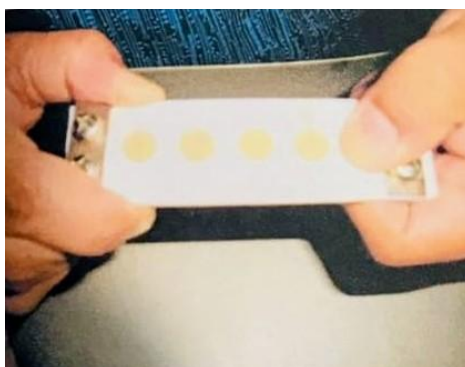
Figure 1: Compression of Giomer Specimen Using Glass Slab in Teflon Mold
