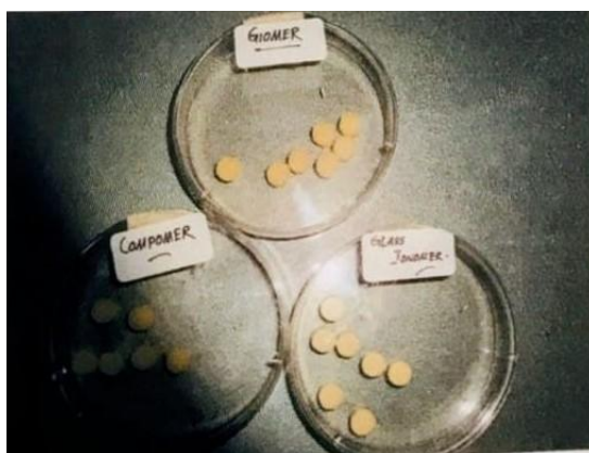
Figure 2: Cured Glass-Ionomer Specimens Prepared for Fluoride Release Assessment
