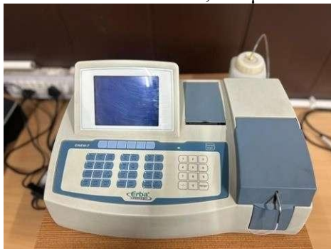
Figure 6. Enzyme activity determination using an ERBA semi-autoanalyser
